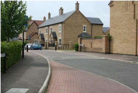
Variations in surface material and raised tables to encourage users of roads to use caution and slow down
